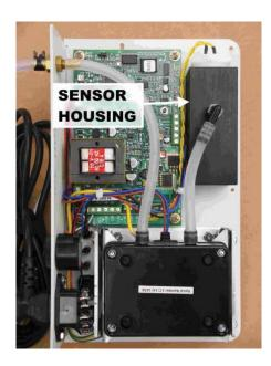
most users, an annual sensor replacement can assure good operation of the monitor. It is recommended to replace the sample tubing and air filter whenever the sensor is replaced.
