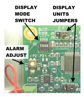
The 8072A is factory set to display dew point in °F. The display can be changed to °C by jumper configuration. With the 8072A panel removed from the carrying case, locate the configurable parts near the upper left corner of the PC board. Move J6 and J7 jumpers to the C position to display dew point in °C.
