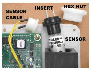
with gasket. The sensor will then unplug from the insert. Replace sensor and inspect gasket for damage. Reassemble all parts, hand tighten the hex nut, and plug in the cable connector.
