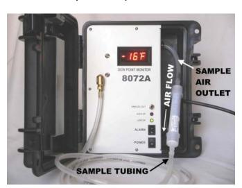
save them for reuse. Connect the sample tubing to one end of the desiccant tube, and the sample air outlet to the other end. This will create a closed loop of dry air flow
